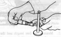
EM030 Fig. EM-25 Measuring Valve Stem Diameter
