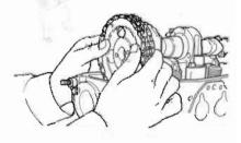
EM707 Fig. EM-6 Removing Camshaft Sprocket
