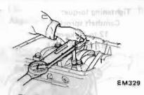
Fig. EM-74 Installing Connecting Rod Cap
